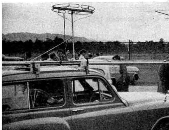
G3FIB/M's 2 metre "halo" aerial aroused considerable interest at the West Kent Radio Society's Mobile Rally at Tonbridge on September 16. It consists of a pair of folded dipoles fed with 300 ohm ribbon and was designed by G2HGR.
